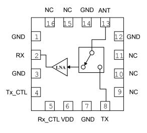
QFN 16 pins, 2.5 x 2.5 (mm)
